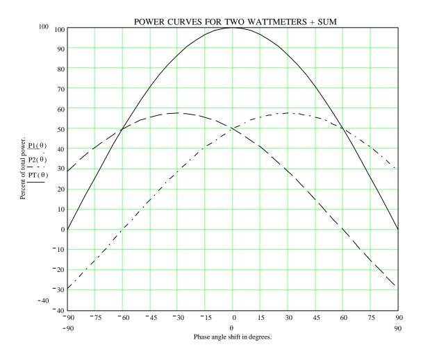
In the graph above the solid line represents total power. The dashed line represents the power as measured from phase A to phase C. The dash-dot line represents the power as measured from phase B to phase C. Some things to note:
