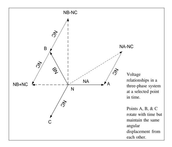
The vector diagram above illustrates the phase relationship in a three-phase system. Note the following:
